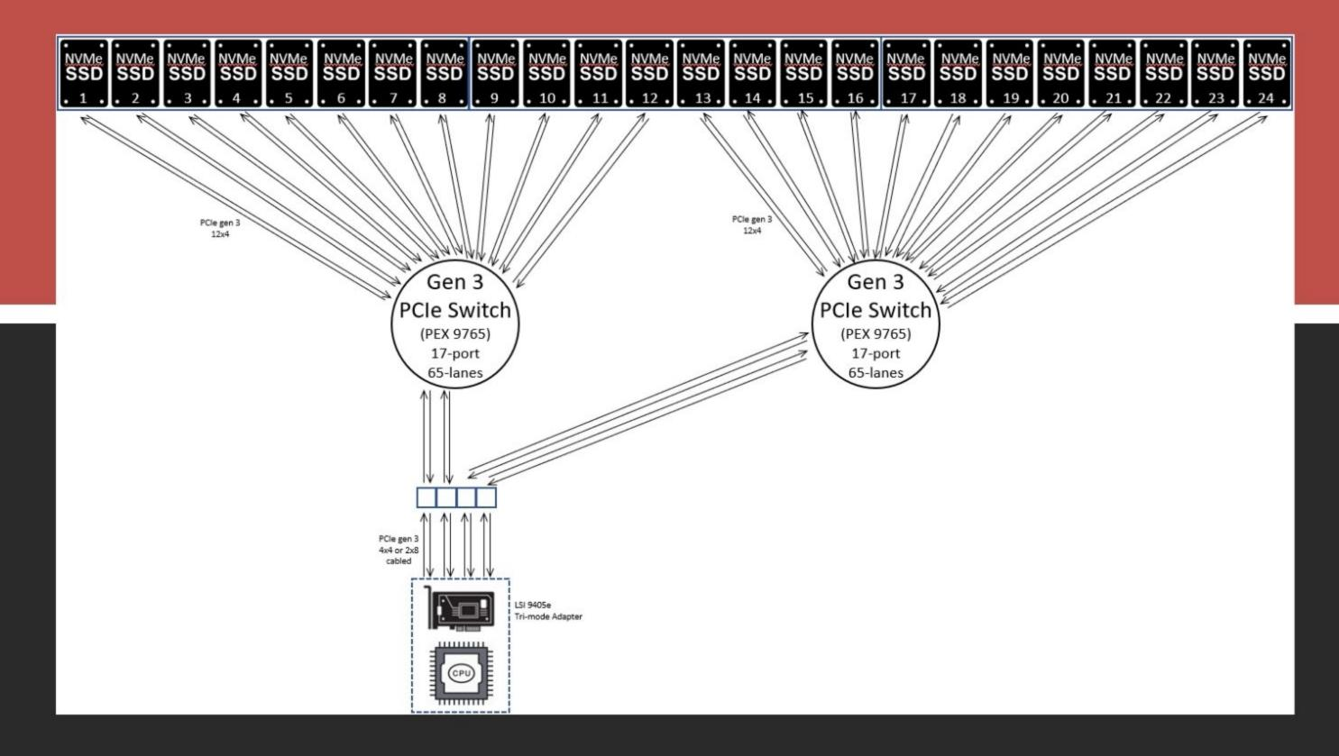
There are several other use cases for the Trenton Systems JBOF System. Here you can see an example where the host computer only has one PCIe expansion card. While not as ideal for bandwidth or redundancy, this lowers the total cost of the system.
